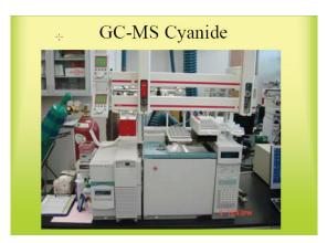
Figure 4. A gas chromatography-mass spectrometry (GC-MS) apparatus used to determine cyanide concentrations. Image provided by Dr. David Klein, Texas Department of State Health Services.
