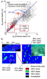
Figure 4: Goodman and Ustin (2007) model applied to CASI data showing: a) Comparison of model derived bathymetry and *in situ* soundings using Pearsons correlation; results of Stumpf et al. (2003) model applied to QuickBird also shown for comparison; and b) False color composite at differing resolutions with percentage coral, algal and sand in the red, green and blue channels respectively. Image typical of patches shown in upper right.
