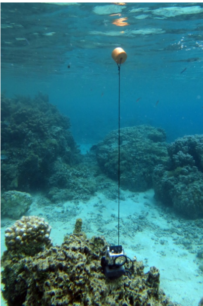
Fig. 5. A GO-Pro video camera deployed on a shallow lagoonal reef in Rangiroa.
