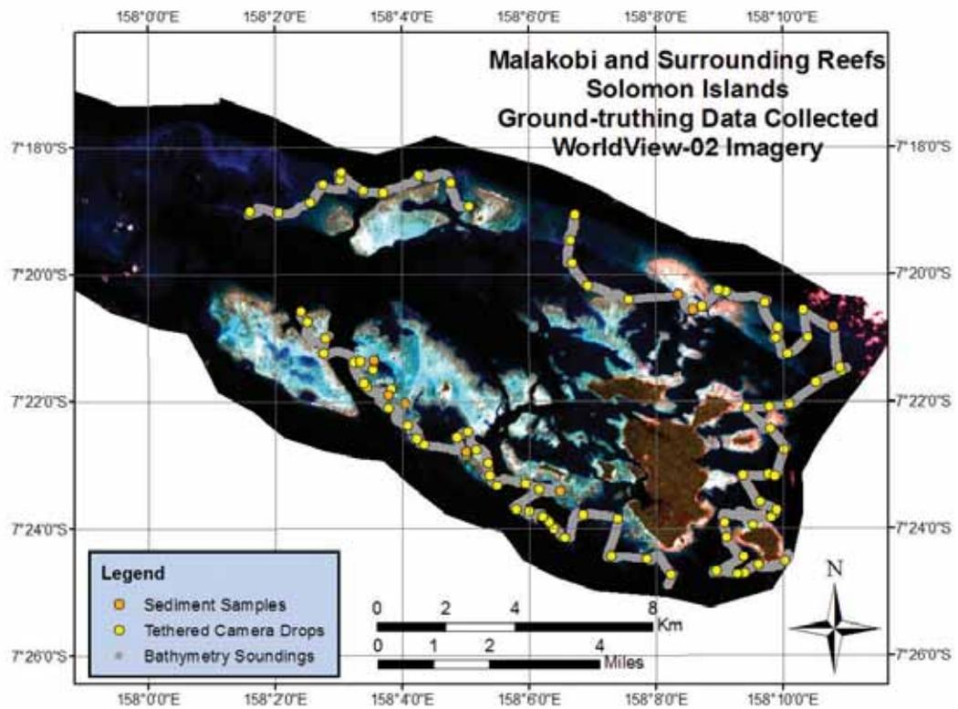
Fig. 18. Track of the research vessel illustrating the locations of bathymetric soundings, drop cameras and sediment samples for Sikopo, Kerehikapa and Malakobi.
