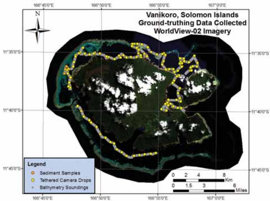
*Fig. 20. Track of the research vessel illustrating the locations of bathymetric soundings, drop cameras and sediment samples for Utupua and Vanikoro.*
