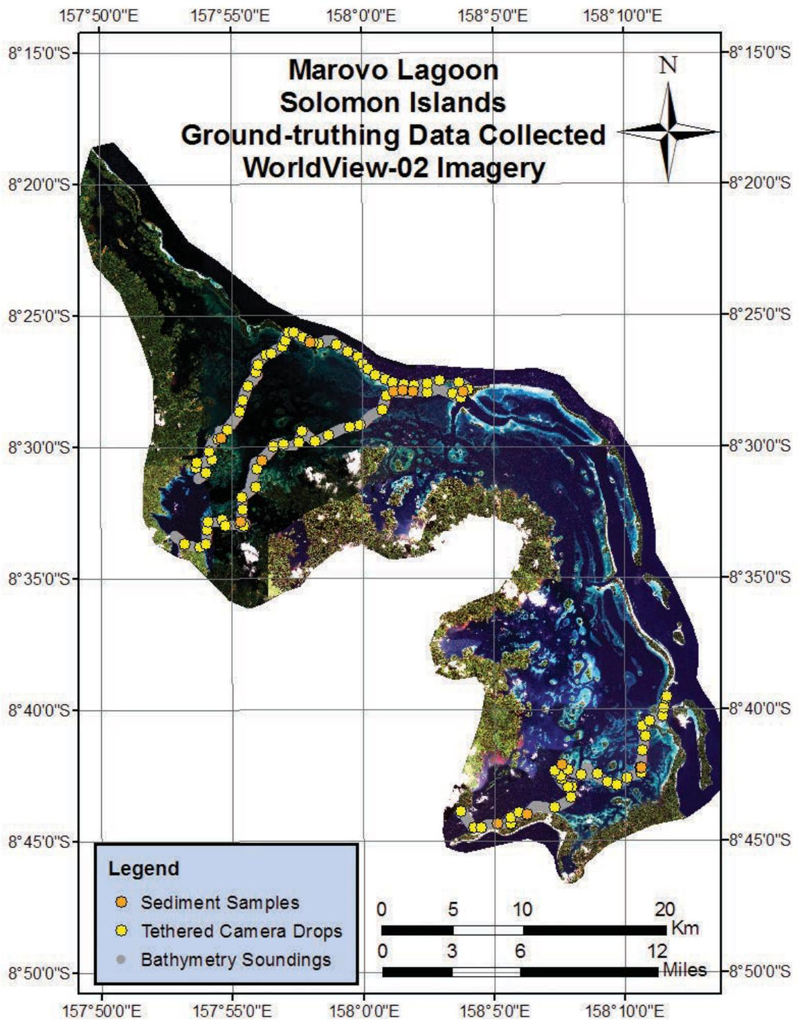
*Fig. 19. Track of the research vessel illustrating the locations of bathymetric soundings, drop cameras and sediment samples for Marovo Lagoon.*
