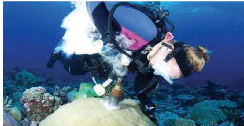
Fig. 27. Removing a core from *Porites lobata* using a pneumatic drill.
