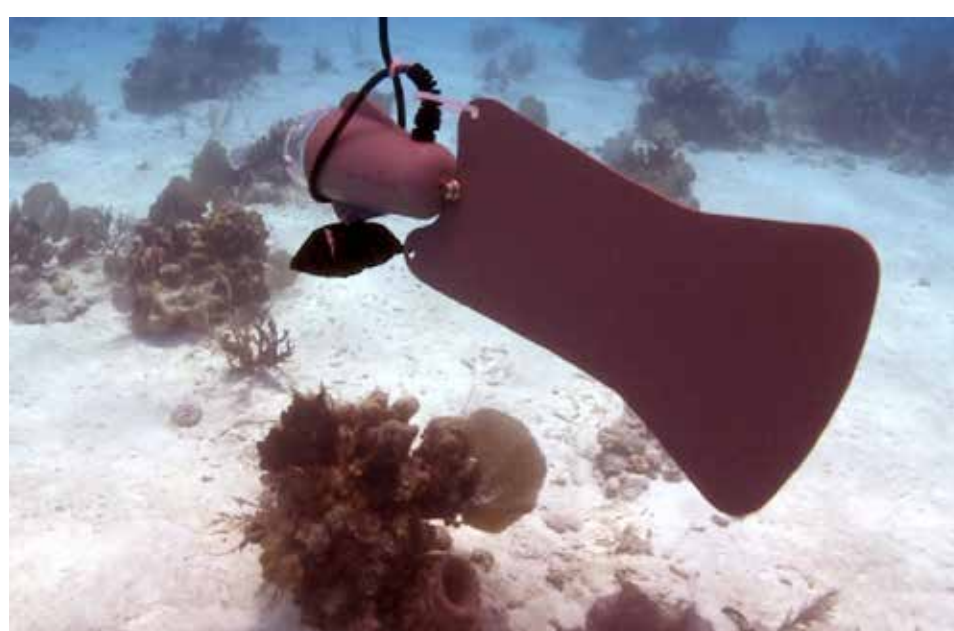
SeaViewer tethered video camera used to characterize habitats. Deploying the tethered video camera (top right); sideview, underwater (right center); and the camera being "flown" above the reef (bottom right).
