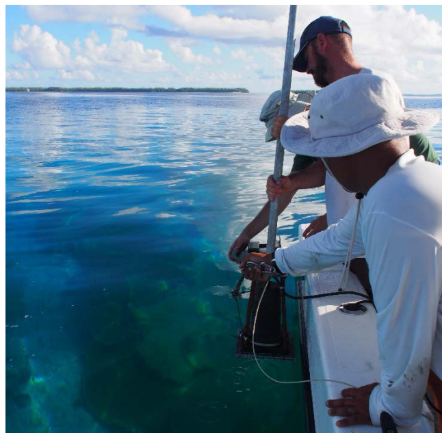
Fig. 33. Deploying the Stratabox at Peros Banhos to identify potential Pleistocene reef structures below the lagoonal sediment.
