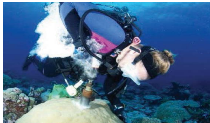
Fig. 47. Removing a core from Porites lobata with a pneumatic drill.
