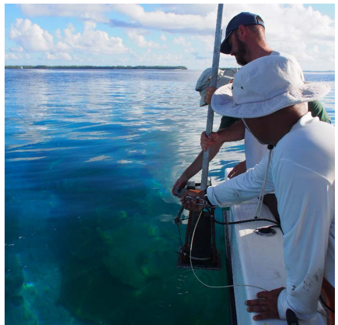
Fig. 33. Deploying the Stratabox at Peros Banhos to identify potential Pleistocene reef structures below the lagoonal sediment.
