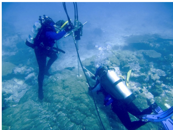
Fig. 51. The drill apparatus on a Porites colony. Image by Konrad Huguen.
