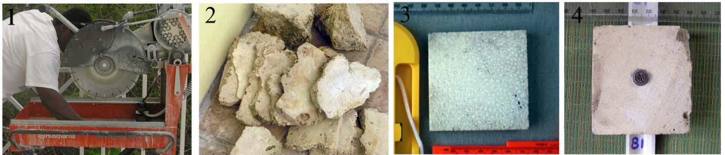
Fig. 36. Masonry saw used to cut the coral fragments, (2) transversal sections of the coral fragments, (3) tile photographed with a size reference, (4) tile attached to the PVC rack for preconditioning.
