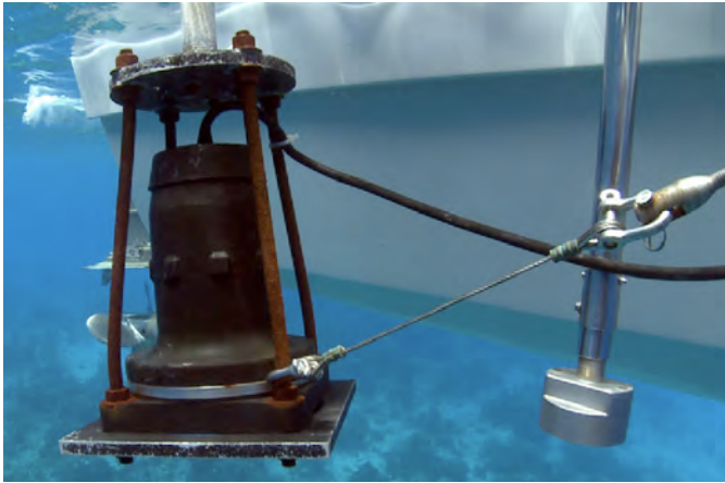
Fig. 2. Acoustic sub-bottom profiling equipment. Stratabox (left) and Hydrobox (right).
