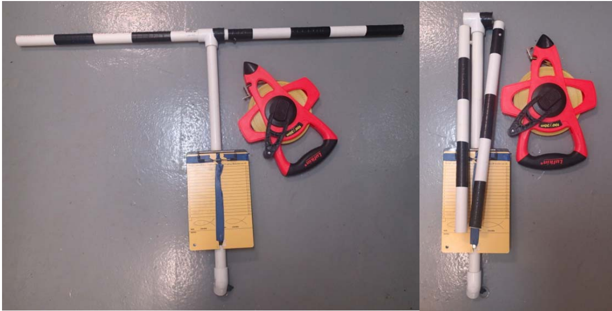
Fig. 36. T bar with attached slate and transect line for fish surveys. The PVC bar is marked in 10 cm intervals with electrical tape. The PVC pipes are connected with bungee cords and can be folded up for ease of transport.
