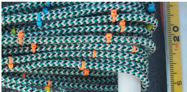
Fig. 23b. Close-up of lead core rope showing the placement of the cable ties at 10 cm intervals.
