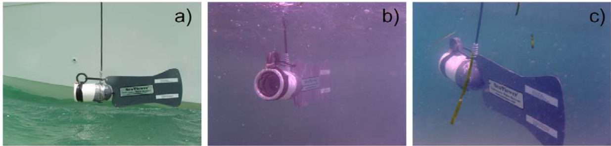
Fig. 5.3a. Drop Camera: The underwater camera is lowered into the water by a reinforced cable. Underwater, the rear fin ensures that the camera flies straight and does not spin, thus producing a stable picture.
